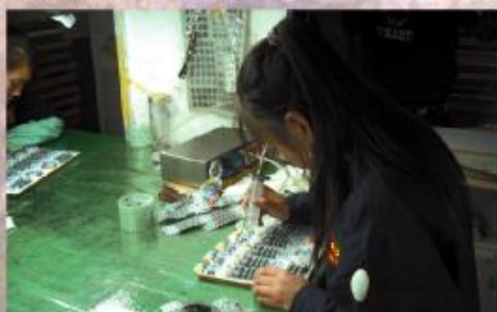
點膠場景 DRIPPING EPOXY VIEW
